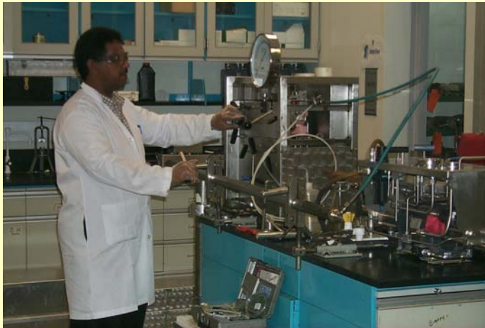
Figure 2. Laboratory Testing of a New Down Hole Sampler
